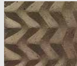
Profile-3D-Printing: Robotic post-processing of 3D printed concrete for geometry actuated thermal performance.
